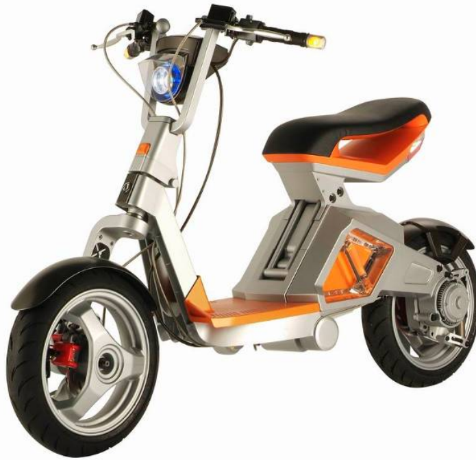
Figure 2: The RoboScooter folding electric motor scooter.
