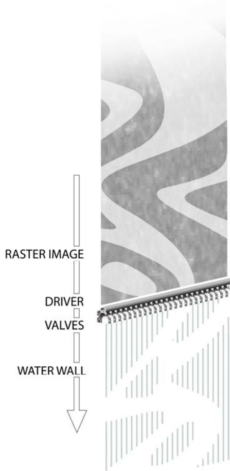
*Creation of a modern, digital Water Wall by computer-controlled solenoid valves.*
