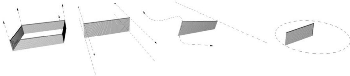
*Water Walls produced by mobile booms can translate vertically and horizontally, rotate, and sweep out ruled surfaces.*
