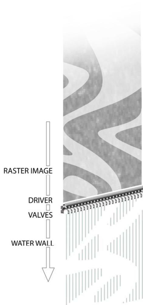
*Creation of a modern, digital Water Wall by computer-controlled solenoid valves.*
