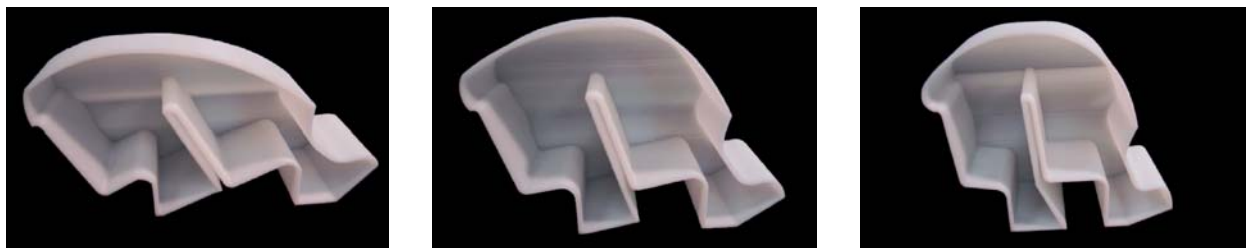
Figure I-19, 20, 21: FDM 3D prints of varying ergonomically defined interior studies
