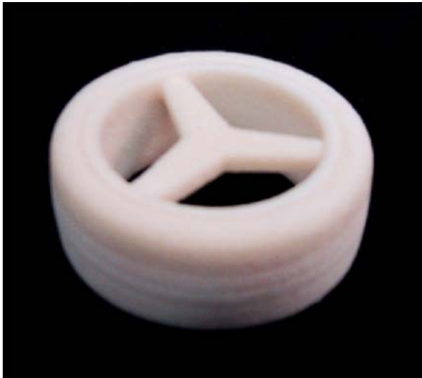
Figure I-10: Z-Corp 3D print of parametric wheel
