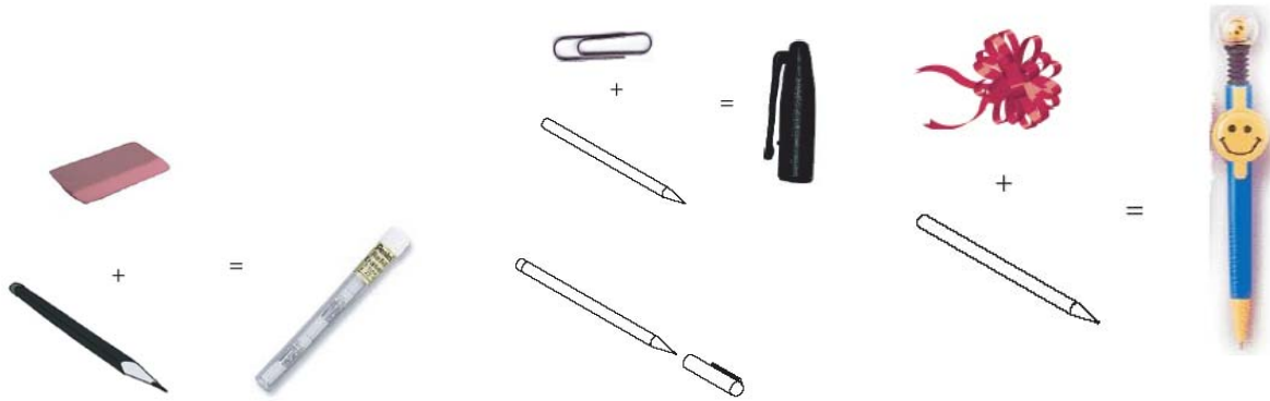
Figure III-15: Introducing additional functions
