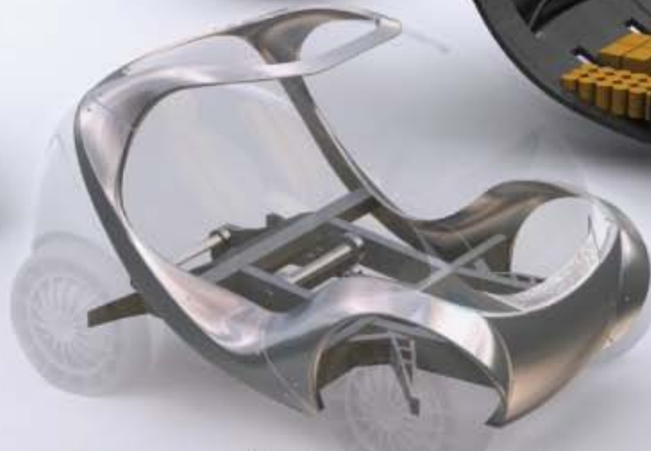
Aluminum Exoskeleton Safety Cage and folding Chassis
