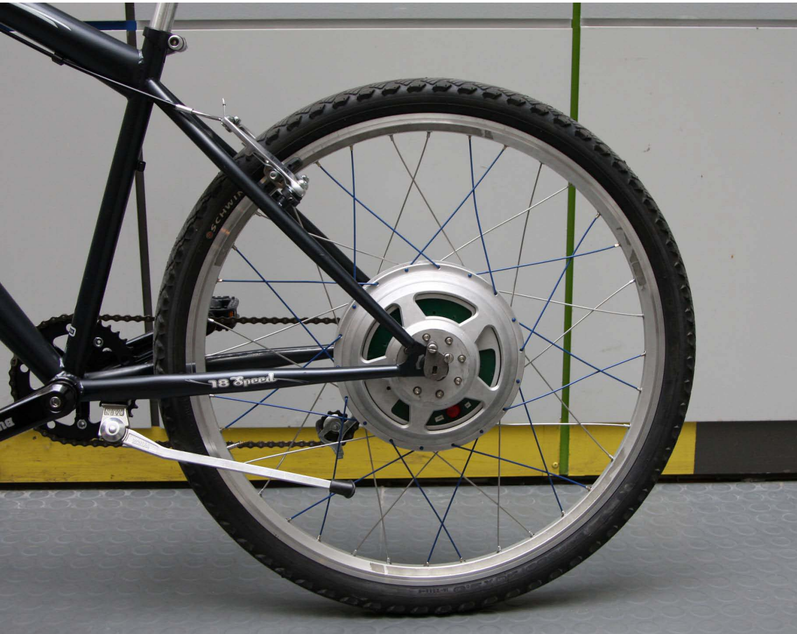
Integrated in-wheel motor and battery hub system
