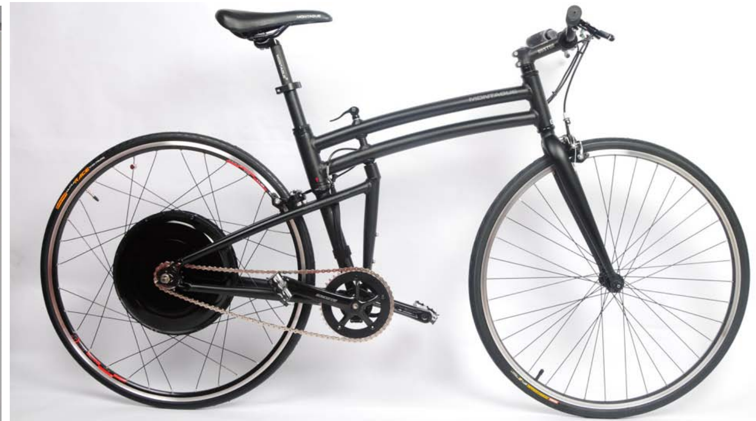
Integrated in-wheel motor and battery hub system
